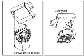
Position housing so that it is centered in existing opening. Make sure housing is flush with finished ceiling or wall. After making electrical connection, driving screws (Ø4×25 mm) through the housing where indicated by arrows.
